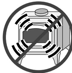
Avoid placing wood against the glass when loading. Do not slam the door or strike the glass.
