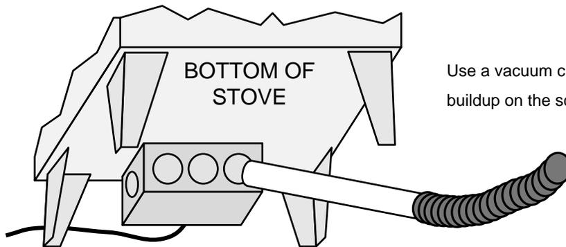
Use a vacuum cleaner to remove any buildup on the screens of the blower.
