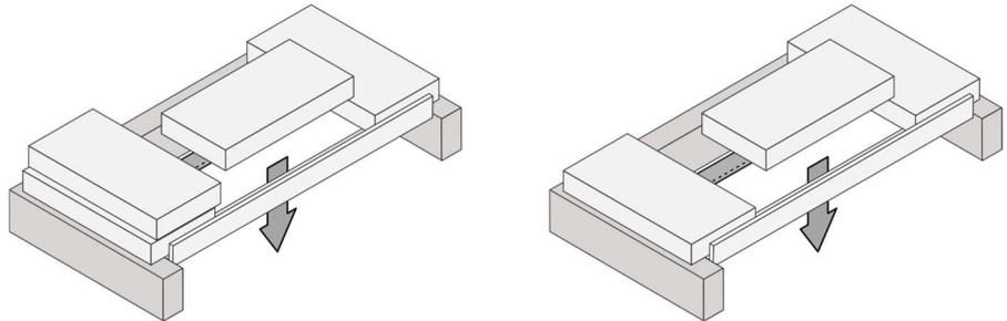
4. Push the two remaining bricks upward until you can rotate them. Lower them past the baffle support and remove them from the firebox.
