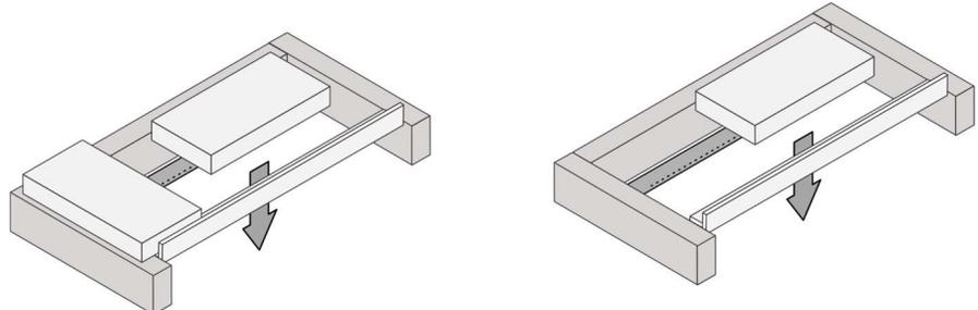
5. Push upward on the baffle support until it is above the side manifolds, rotate it slightly, and remove it from the firebox.
