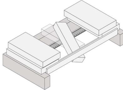
3. Rotate the bricks that were moved aside in step 1, lower them past the baffle support and remove them from the firebox.
