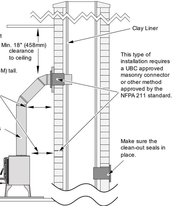
This type of installation requires a UBC approved masonry connector or other method approved by the NFPA 211 standard.
