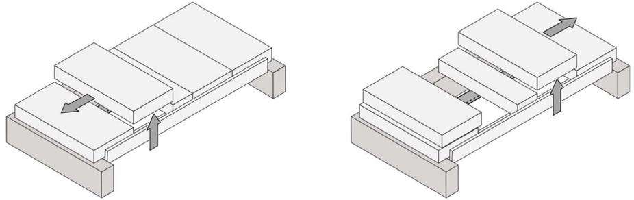
2. Push up on the center brick and rotate it slightly until you can lower it past the baffle support and remove it from the firebox.
