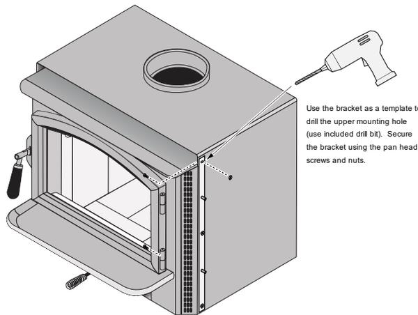
4. Place the insert into position (flue attached). Attach the surround panel as shown below.
